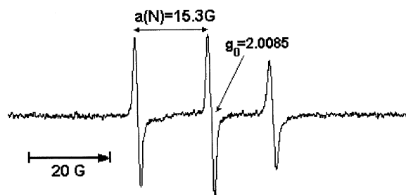
Fig. 2. EPR spectrum of the Tempyo spin label at low pH.
